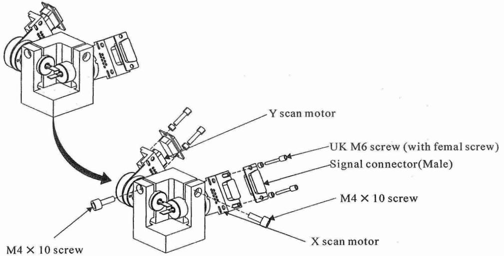
Fig6-1 Scan motor install diagram
